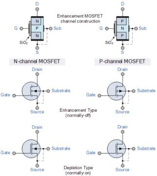
The line between the drain and source connections represents the semiconductive channel. If this is a solid unbroken line then this represents a "Depletion" (normally-ON) type MOSFET as drain current can flow
