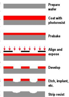
complex structures that make up a transistor and the many wires that connect the millions of transistors of a circuit, lithography and etch pattern transfer steps are repeated at least 10 times, but more typically are done 20 to 30 times to make one circuit. Each pattern being printed on the wafer is aligned to the previously formed patterns and slowly the conductors, insulators, and selectively doped regions are built up to form the final device.
